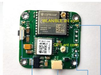
configuration button and LED power connector status LED aux power connector
