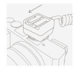
Reach M+ connects to the camera hot shoe port which is synced to the shutter.
