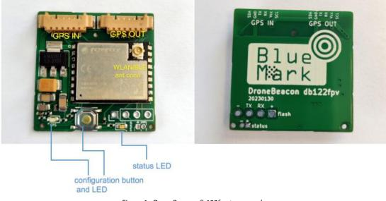
Figure 1 - DroneBeacon db122fpv transponders
