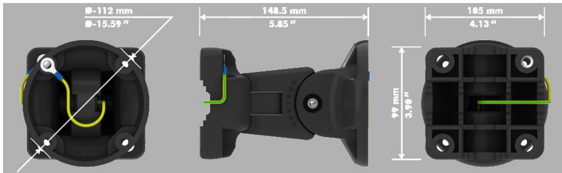
Figure 4 - mast mount to install the receiver to a mast or directly to a wall.
