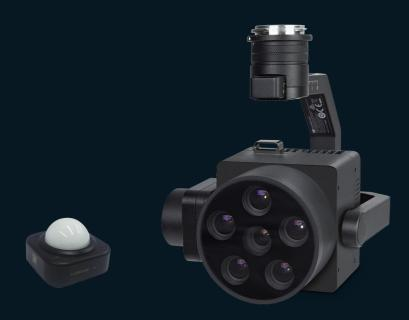
Five 3.2-megapixel multispectral channels and one 12.3-megapixel RGB channel. Sapphire optical window, large aperture, low distortion, broadband projection, all-glass lens and an aluminum alloy camera housing. In addition, AQ600 Pro can transmit spectral remote sensing video and output results in real time, which provides new technical means for precision agriculture, forestry monitoring, river monitoring, ecological protection, target recognition and other industrial applications.
