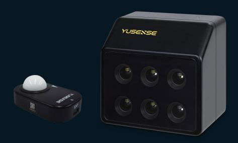
Based on the MS600 V2 multi-spectral camera host, the band configuration is optimized on the basis of maintaining the appearance and main performance of the product, which is consistent with the current mainstream satellite band design such as Sentinel-2 and Landsat-Next. It ensures the information unification of satellite-borne and airborne spectral data by scientific researchers in agriculture, forestry and grass industry, ecological environment and other fields to the greatest extent.
